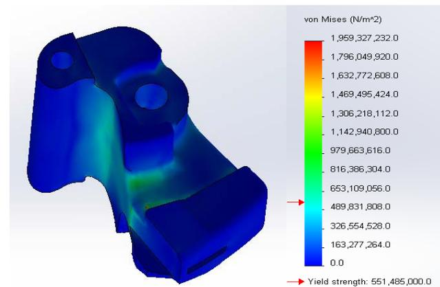
Figure 2(b). FEA of Model without Hinge pin
