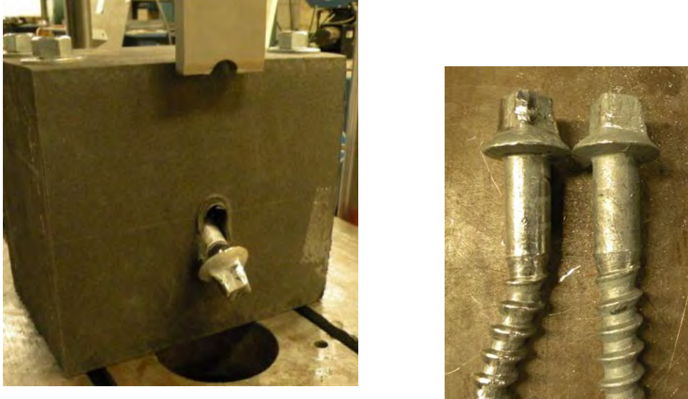
Figure 13. Spike lateral restraint mode of failure.
