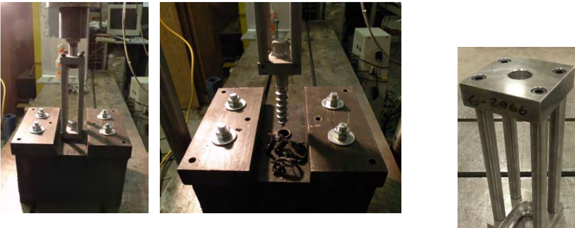
Figure 2. Pullout test configuration, mode of failure and pullout device.
