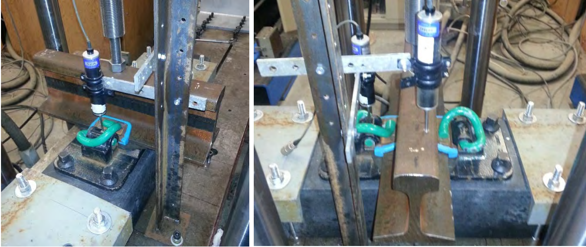
Figure 7. Fastener uplift test setup.
