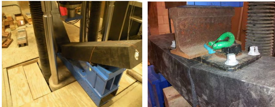
Figure 7. Failure of the center bending test (left) and rail seat bending with the rail (right).
