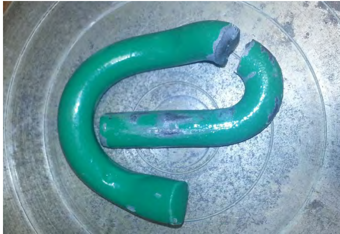
Figure 8. Failure of the fastening clip.
