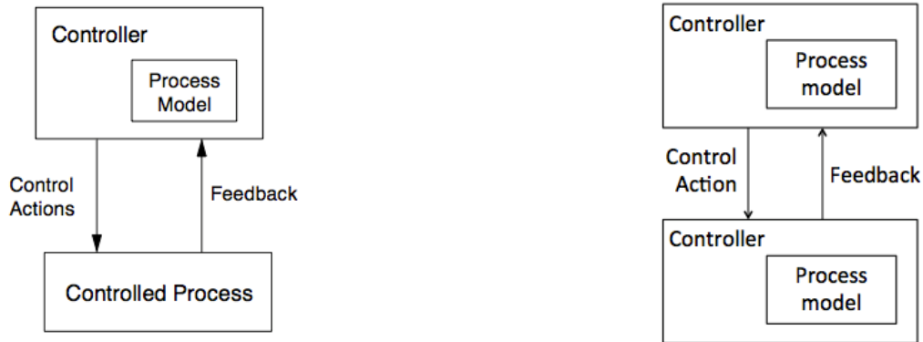
Figure 5-2: Two example of a single control loop: on the left, a controller controls a process and on the right, a an upper-level controller controls a lower level controller (Source: Leveson 2011a [left] and author, adapted from Leveson 2011a [right])
